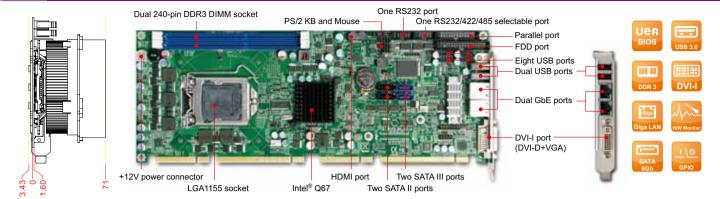
ROBO-8110VG2AR-Q67 is based on the Intel® Q67 chipset and desktop processor sku like Intel® Core™ i7 and i5. Built with flexible PCI express expansion, it's suitable for Medical, Industrial Automation, and Digital Signage applications.
